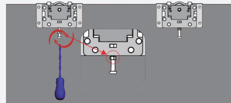
Regulate screw to adjust the gap of door, then fasten it
