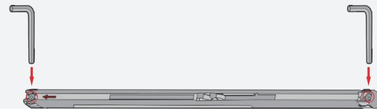
Allen key to fix the damper on the rail
